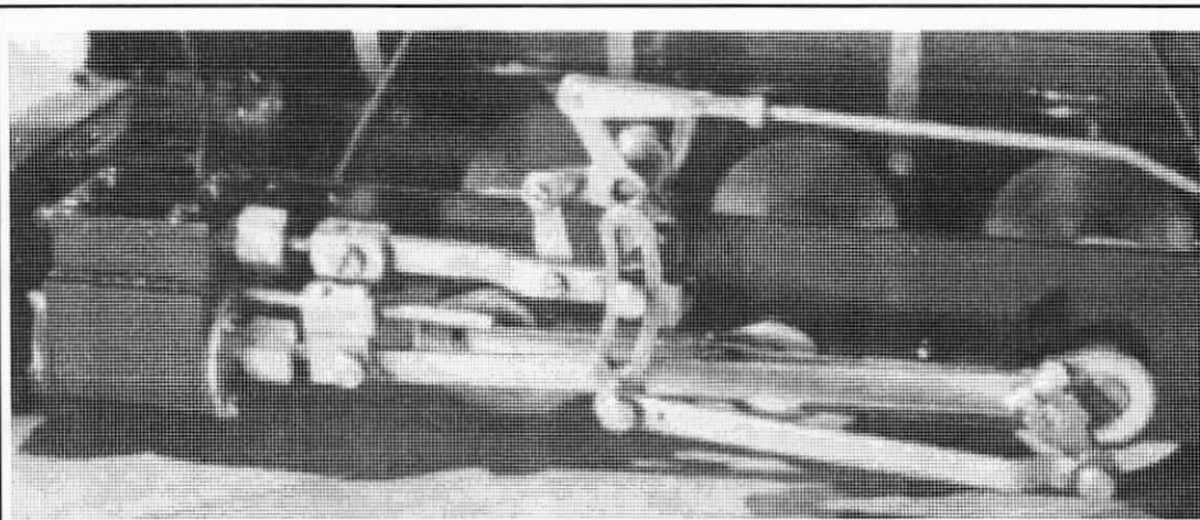
ABOVE: Closeup of the Walschaert's valve gear and cylinders on the Roundhouse Fowler. The link and clevis at the top center is attached to the direction control servo or reversing quadrant in the cab.
