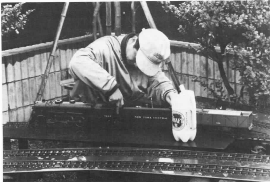
New York Central (Aster), butane fired, on steaming bay. Note the beer bottle. These are used to hold water for firing and emergencies. Red bottles are placed around the tracksite at 3 meter intervals for emergency use.
