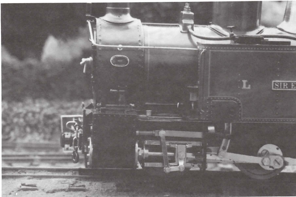
Note the etched brass detailing on the side sheets and the neatly crafted valve gear.
