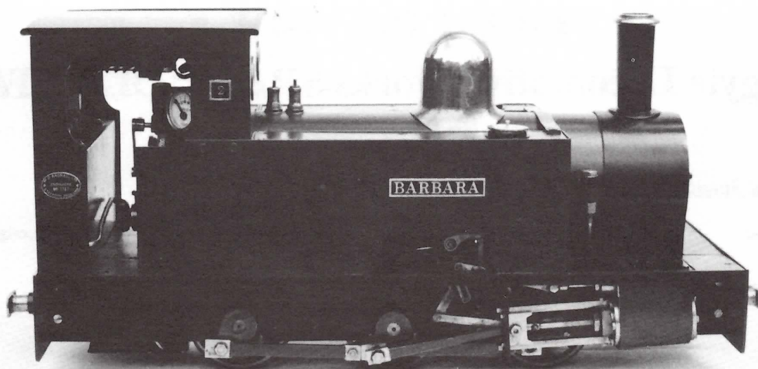
This 16mm/ft. model of Snailbeach District Railways W.G. Bagnall No. 1797 of 1906, "DENNIS", was re-named "BARBARA" to dissuade the owner's wife from asking the cost! The engine is fully sprung, gas-fired, and equipped with Bagnall-Price valve gear. It requires a minimum curve radius of 3'-6".
