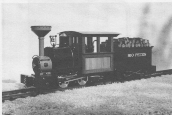
Below: Rio Pecos custom wood cab on Maxwell Hemmens Porter locomotive. Mahogany and white oak construction, with tightly fitted joints.
