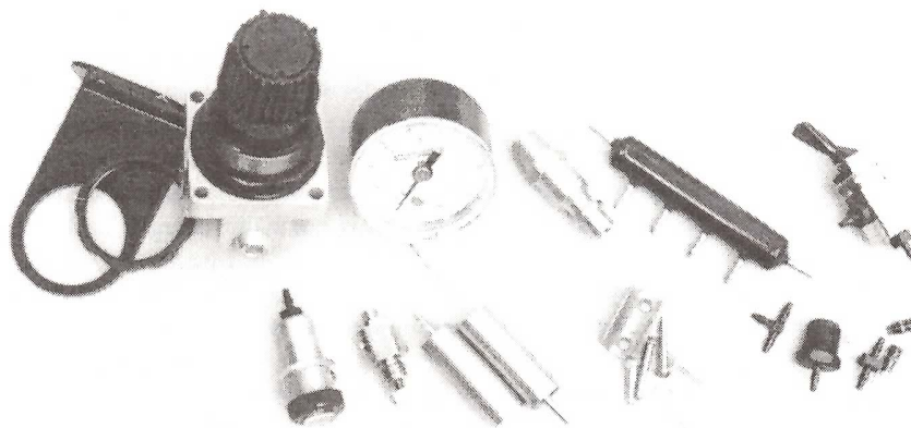
Bits & Pieces -- Back row: regulator & brackets, gauge, quick-connect coupling, manifold and toggle. Front row: indicator, slo-motion control, air motors, mounting hardware, caps, tees, plugs & reducers.
