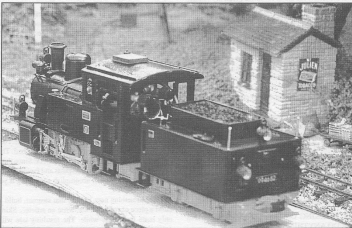
The modified Frank S. Note the gas control valve in the rear window of the cab. The new tank is just visible through the cab doorway, and you should see the filler on the front of the side tank. Currently awaiting new nameplates, this engine will be named Wermland . Note also that the tender now boasts a coal load.
