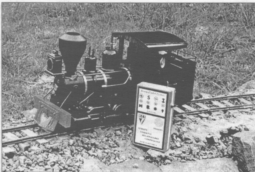
Here you can see the layout and the very compact size of the RCS transmitter. Also note that there's no long antenna to poke out your eyes or get caught in the shrubbery.
