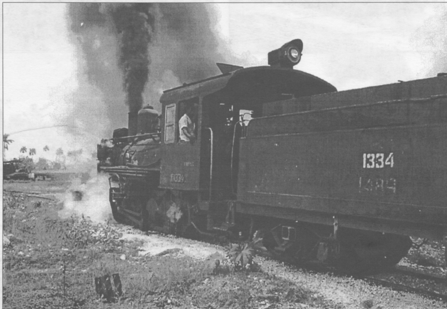
At the Obdulio Morales Mill, Nº 1334, a 1920 Baldwin 2-8-0, belches clouds of thick, black smoke as it hauls loads of sugar cane on 2' 3-3/4" gauge rails.
