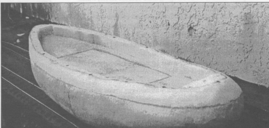
The same hull as in the preceding photo, but with bulwarks attached. Nails, rather than glue, was used to attach the bulwarks.
