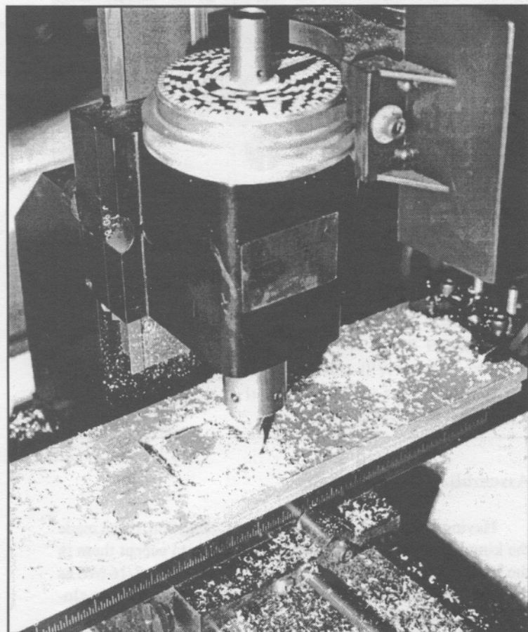
Milling out the aperture for the Graham twin in the 1/4" aluminum plate. The plate is supported on a sacrificial piece and milled right through.
