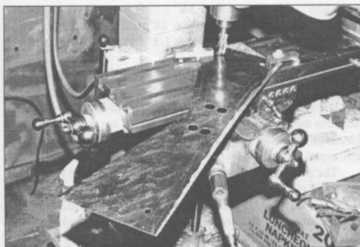
Fabricating the sheet metal which will become the support for the propeller mounting.
