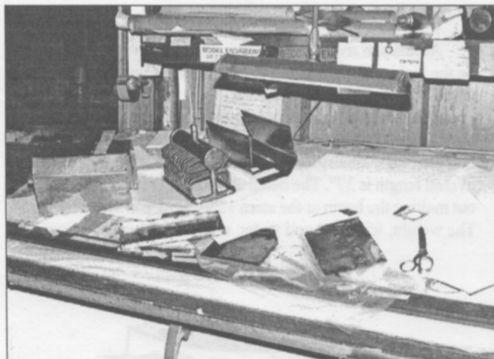
Boiler casing under construction; outer shell is made of stainless steel. Thin metal inner shell with 1/8" insulation between shells.
