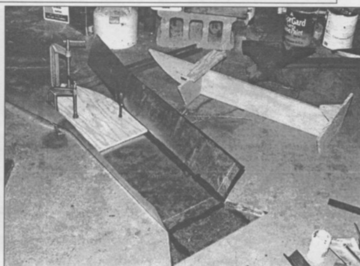
Both sides are formed up, the wood form is clamped in place and the tabs for riveting will be formed up next.
