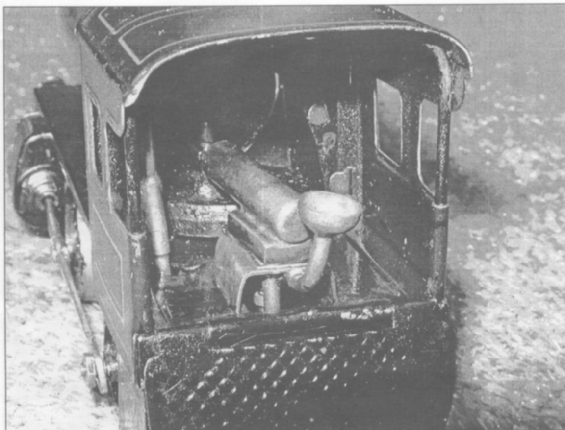
Closeup of the single oscillating cylinder that powers Jim Montgomery's antique Bing gauge 0 steam loco.
