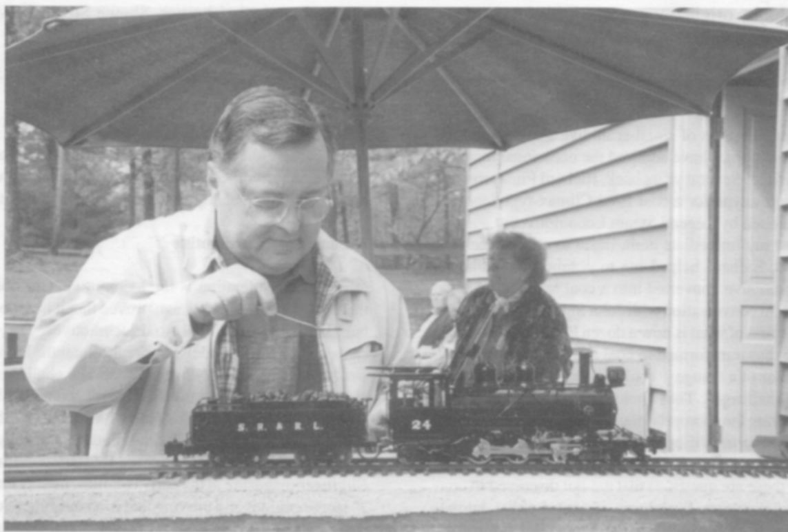
Building a fire on a fall afternoon, Jim Pitts of Travelers Rest, SC steadies his hand as he begins to shovel charcoal in the firebox of his Roundhouse/Shawe SR&RL #24. Real wood charcoal soaked in lamp oil provides the base for a coal fire.
