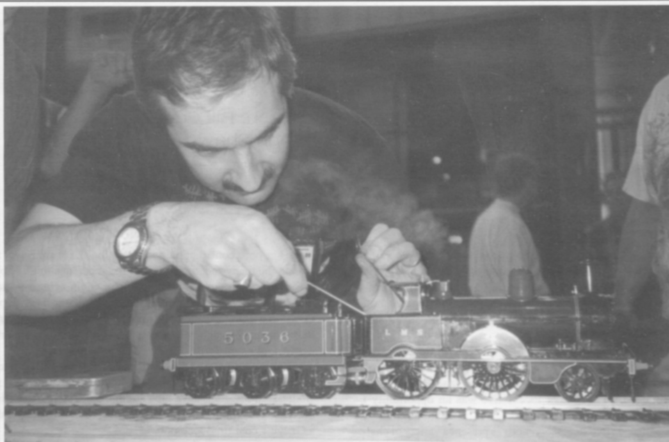
John Shawe, a UK locomotive builder, demonstrates the fine art of coal firing on a converted 2-4-0 JUMBO. Aster Hobby originally produced this LMS crimson red model as an alcohol burner. Shawe Steam Services specializes in custom built as well as coal fired conversions.
