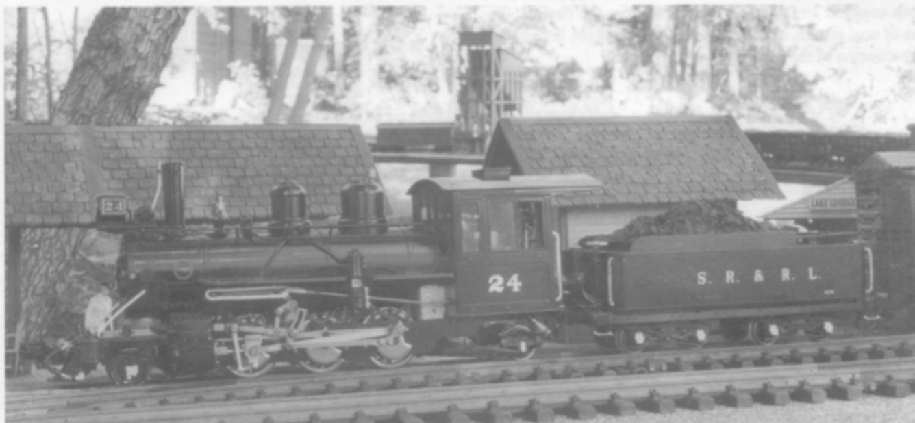
Originally built for Maine's two-foot gauge Sandy River and Rangeley Lakes Railroad, the SR&RL #24 prototype was over 46 feet long. One of the larger Roundhouse locomotives, it offers the bulk and mass that easily accommodates a coal fired firebox, boiler and axle pump. Like the original N o 24, approximately a dozen of these Gauge 1 locomotives are now coal fired.
