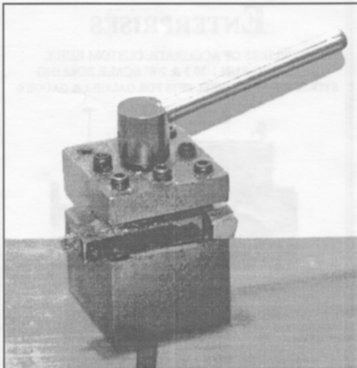
Author's 4-way toolpost mounted on his Peatol Microlathe.
