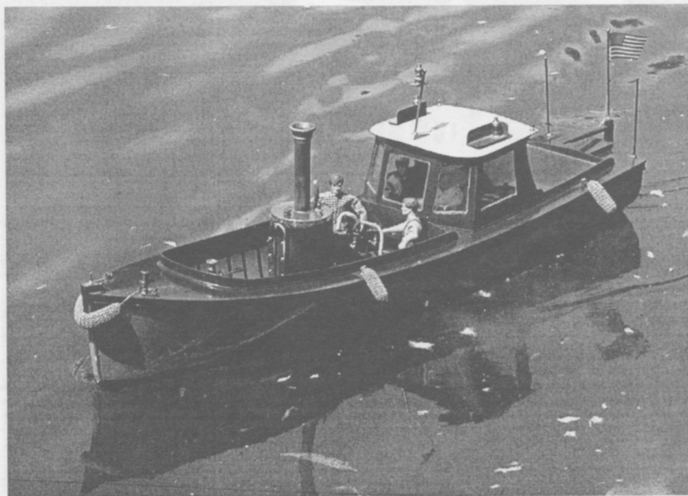
Photo - above: Faithful Assistant gathers information on the tug Imara , built by Ray Suder of Pennsylvania. The hull is fiberglass, 43-1/2" in length, and the completed model weighs in at 32-1/2 lbs.
