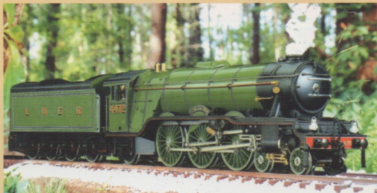
LNER A3 FLYING SCOTSMAN, ALCOHOL, GRESLEY 3 CYL. CONJUGATED VALVE GEAR
