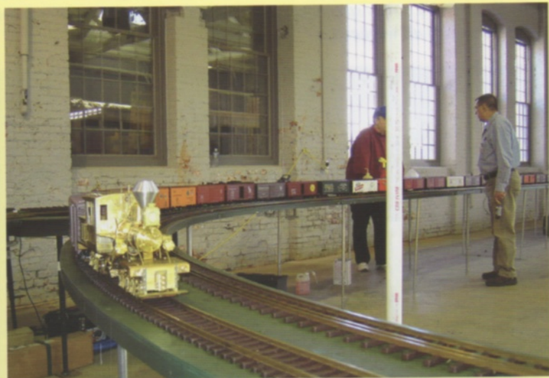
Mike Moore suggested that this would be a good venue in which to test the pulling power of the new Catatunk Climax. It never did run out of power, but ran out of traction on the oily rails at 41 cars.
