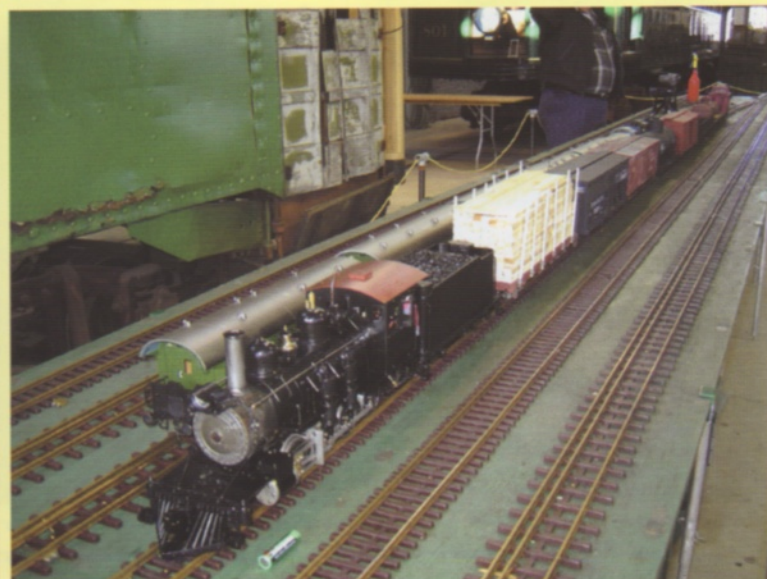
Noel Crawford's loco running on propane power. The gas cylinder and regulator are hidden under the dummy lumber load.
