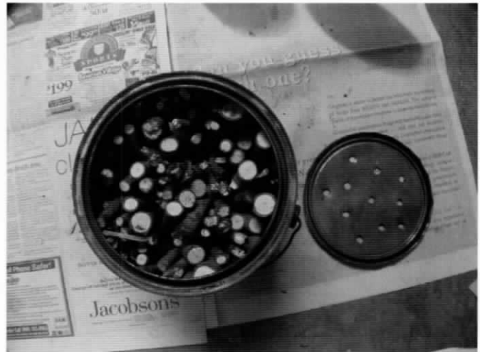
Sticks packed in can and ready to convert to charcoal.
