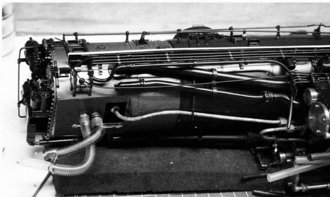
New steam and exhaust piping going towards the front engine (note the absence of the second pipe coming through the cheater hole in the smokebox), which will be insulated for heat conservation.
