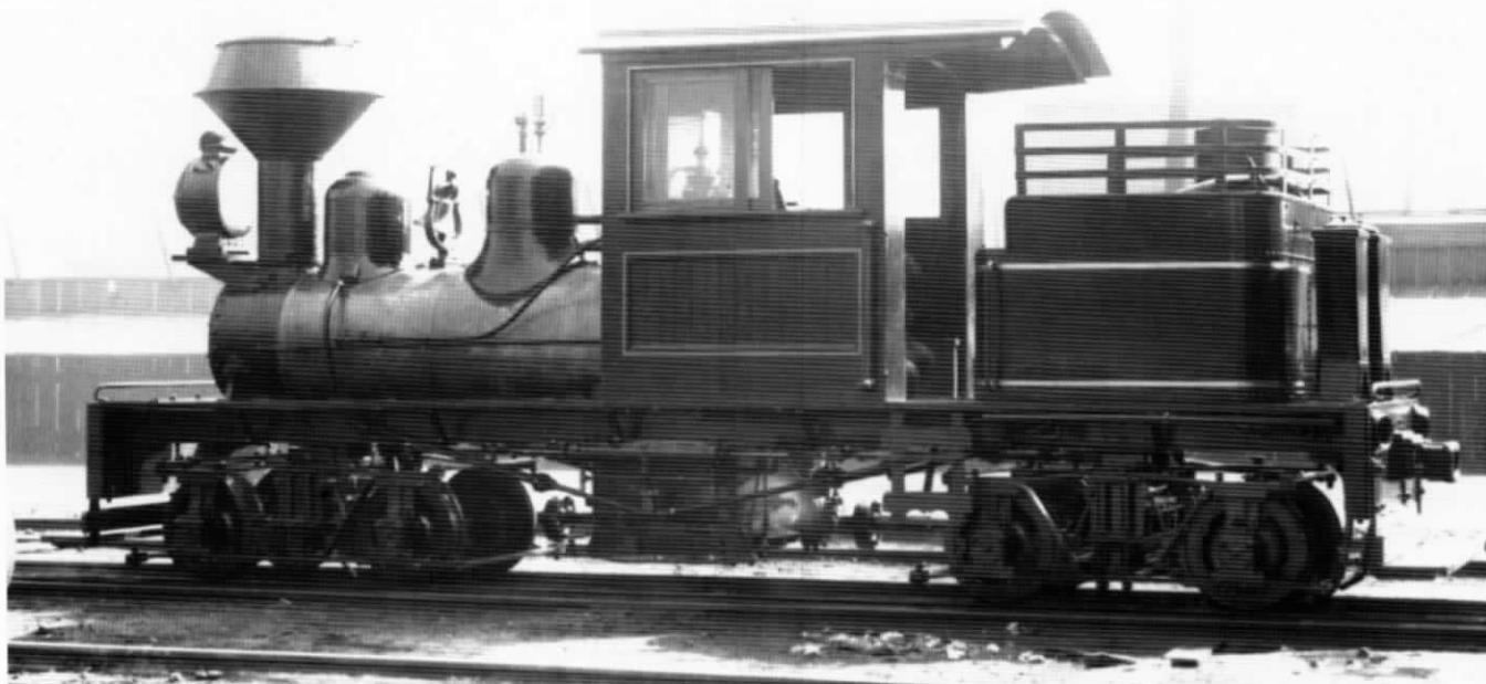
Shop Number 2295 is a 3 foot gauge wood burning Shay built to Plan 1553. Photo courtesy Allen County Historical Society Lima OH
