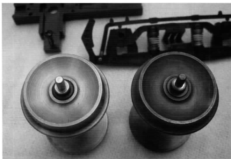
Wheelsets before and after blackening.
