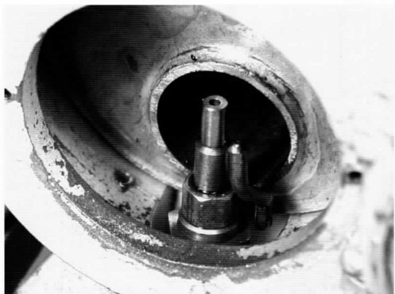
Blast pipe and blower in smokebox.
