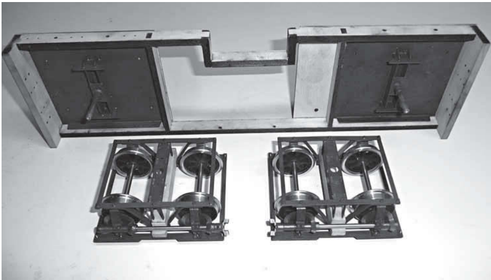
The assembled trucks and frame with metal truck mounting plates in place.
