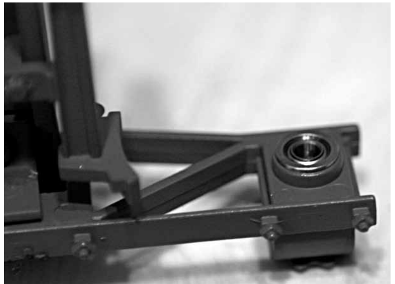
Ball bearings decrease rolling resistance dramatically.
