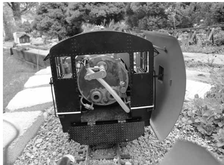
Above Two views of the backhead. The blue tube, which appears here in storage position, supplies the tender bath area with water from the boiler. Directly above this tube is a hand operated valve activated by pressing it downward. The reverser lever is on the right with room behind it for an R/C servo. The throttle is near the top of the backhead, here with an R/C lever attached. On top of the boiler is the water filler plug.
