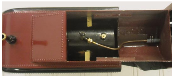
Fuel details: The rear bunker with the coal load removed shows the fuel tank. The fuel valve comes up through the coal load so it can be adjusted mid-run. The stack in the back is the rear-engine exhaust.
