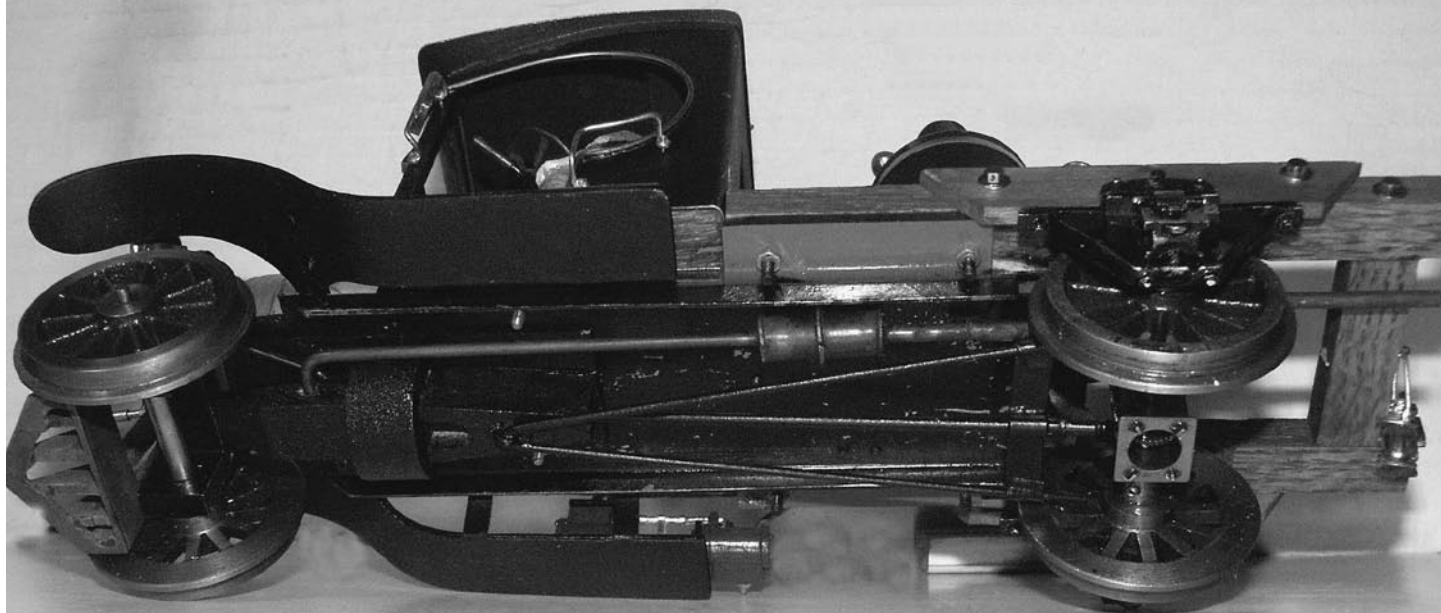
Undercarriage: The Model-T rail truck has details on the underside, including a muffer and muffer pipe.
