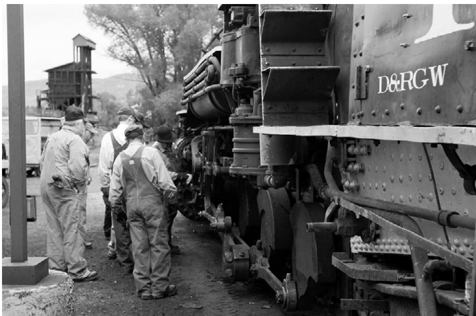
Oiling, greasing, checking: The class gathers around as various external components are checked, oiled and/or greased.
