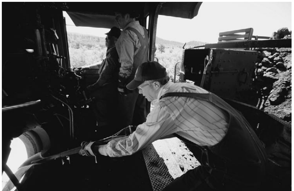
Shoveling as fast as he can: The author learns the finer points of getting the coal as far to the front of the K-36's firebox as possible.
