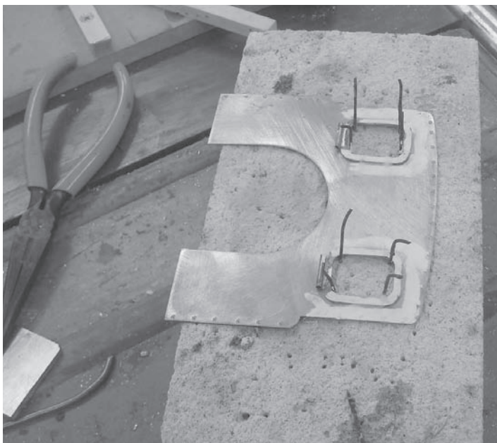
Cab: Left, window frames ready to be soldered. Right, window frames gang-clamped in the mill vise.
