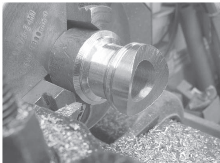
Door and dome: Left, the smoke box front was machined from disks of brass; it is in two major pieces — the door and the outside fixed portion. Above, domes were machined from round stock, which was then chucked in the lathe.
