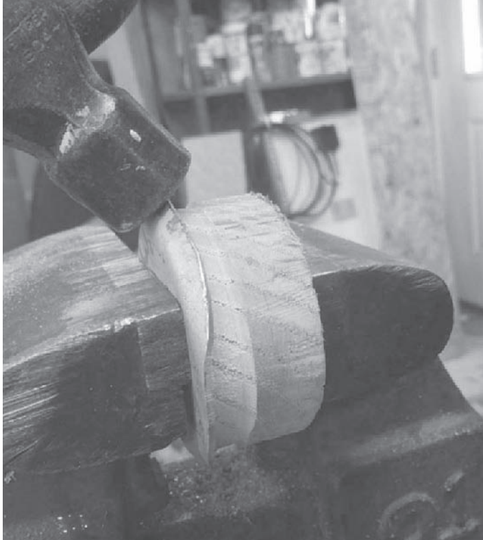
Boiler fab: Left, a boiler end cap is formed from flattened copper pipe with a hammer and hardwood die. Right, holes were drilled in the smoke box and brass escutcheon pins are used to simulate rivets.
