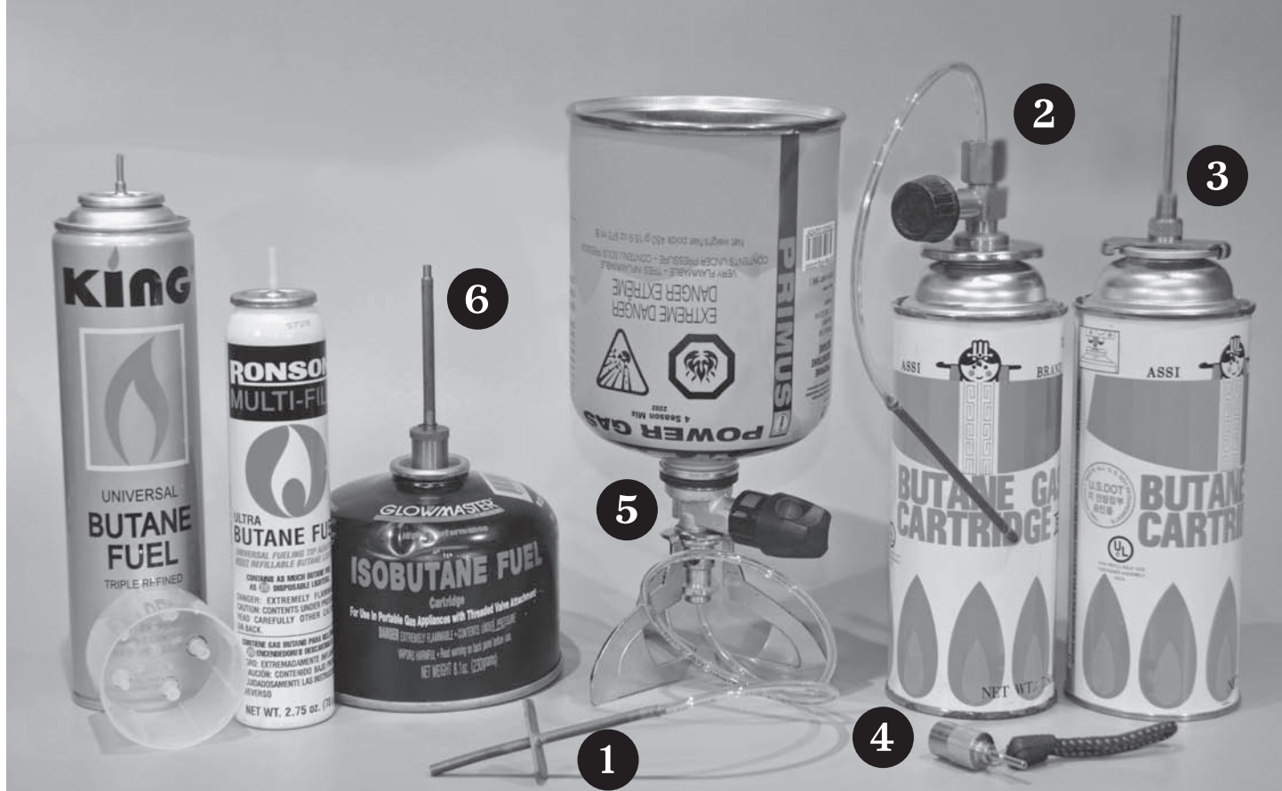
Gas containers, fillers: Left, King Butane Fuel, with built-in nozzle and extra fittings in cap. Next left, a can of Ronson fuel. 6 Isobutane can with common screw-on adapter. 5 Primus can with stand and valve hose. 2 Korean can with valve, hose, adapter. 3 Korean can with collar, adapter. 4 Primus screw-on adapter with lanyard. 1 Modified Accucraft adapter.
