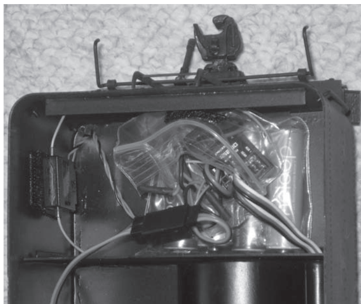
Bagged: The R/C gear in its plastic bag. The second antenna of the AR6200 is attached with Velcro to the side of the box.
