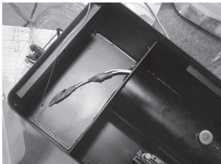
Tender: Rear compartment of tender, with two servo extenders pulled through with fishing line.
