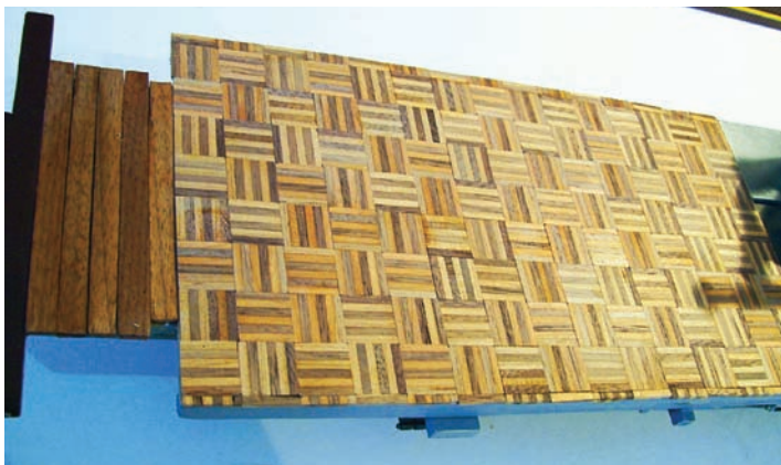
Floor: The parquet floor used on the drawing room and galley half of the car.
