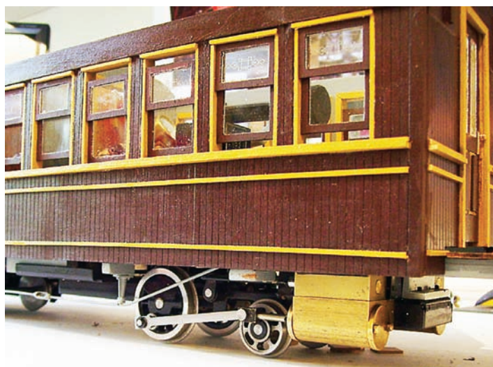
Power and guidance: The car has a single drive wheel with a single leading truck.
