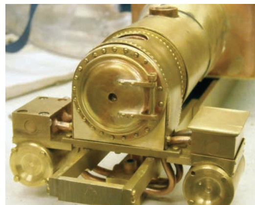
Wrap, smokebox: Left, soldered boiler has wrap attached. Right, smokebox front detail and S-shaped tubes.
