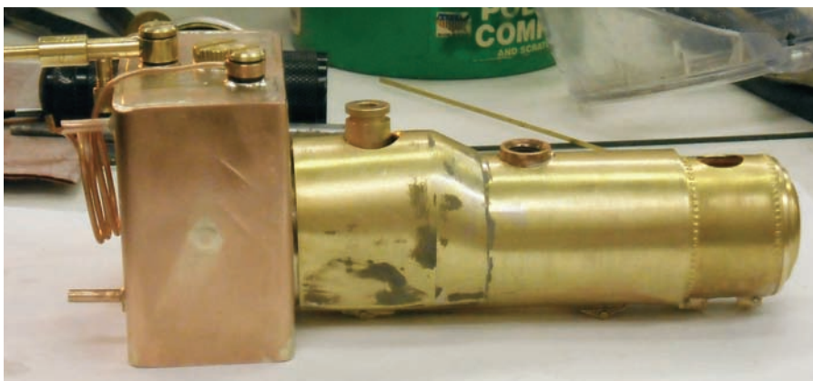
Wrap, smokebox: Left, soldered boiler has wrap attached. Right, smokebox front detail and S-shaped tubes.
