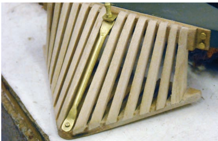
Front, back: Left, cow catcher shows interlocking joints. Right, bunker was formed from brass.
