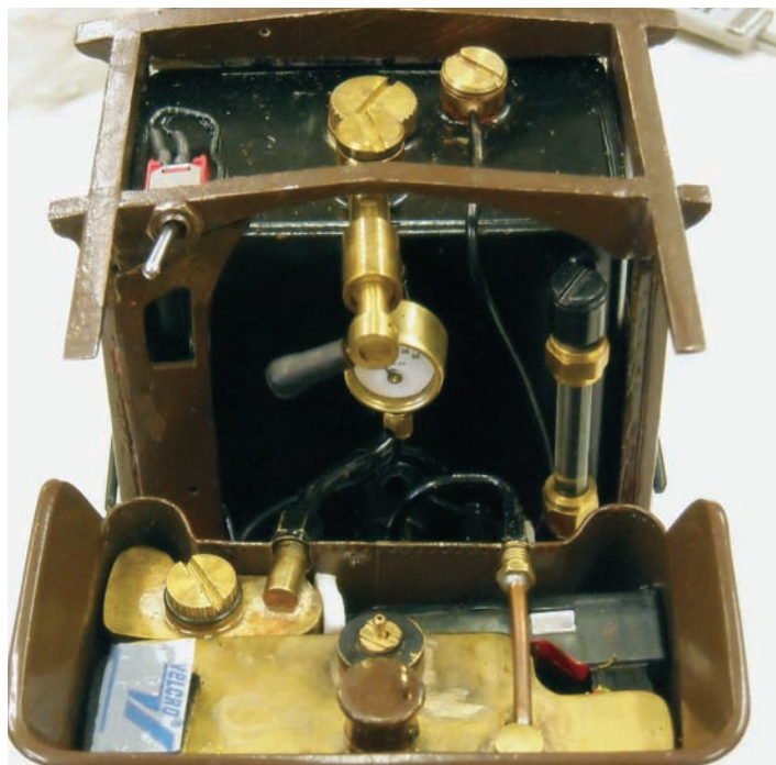
Controls: At the top, the on/off switch for radio control; the throttle is in the center above the pressure gauge, and the sight glass is on the right. In the bunker, lubricator is left front, RC receiver right front and fuel tank in the rear.
