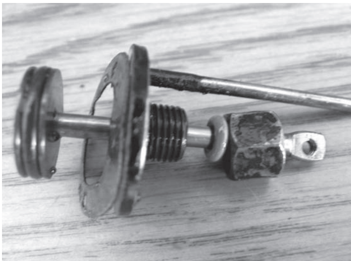
Breakdown of a potential problem: Left, piston, piston seal, rear cylinder head, rear cylinder head paper seal, piston rod and gland seal. Right, rear cylinder head and paper seal.
