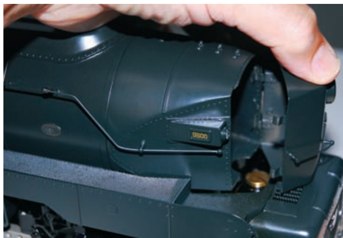
Fittings: Upper left, a wrench tightens the water-supply nut. Lower left, the coal load taken off the tender shows the alcohol and water tanks. Above, the smoke box door opens to reveal extra space.
