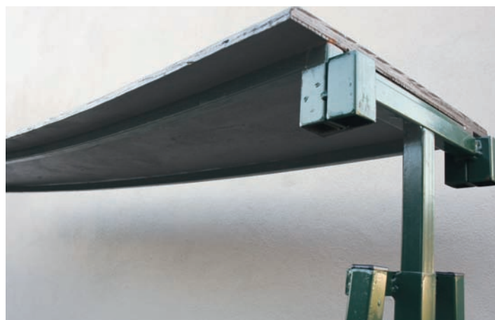
Connections: A flange on the layout deck fits inside the legs' square tubing, with each leg having four flange receptacles. Photo by Rich Jacobs.
