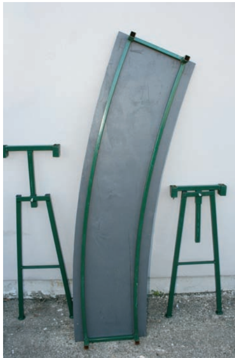
Legs, deck: Welded square tubing is used for legs and deck support on the new track layouts for the Diamondhead steamup. Photo by Rich Jacobs.
