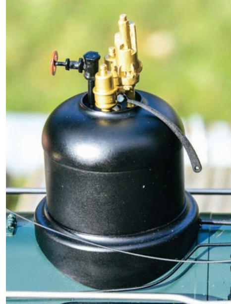
Back head to dome: Left, the C-25 requires removing the cab roof to access the back-head controls. Right, the steam dome has a number of nice details, including a steam-relief valve and an imitation whistle.
