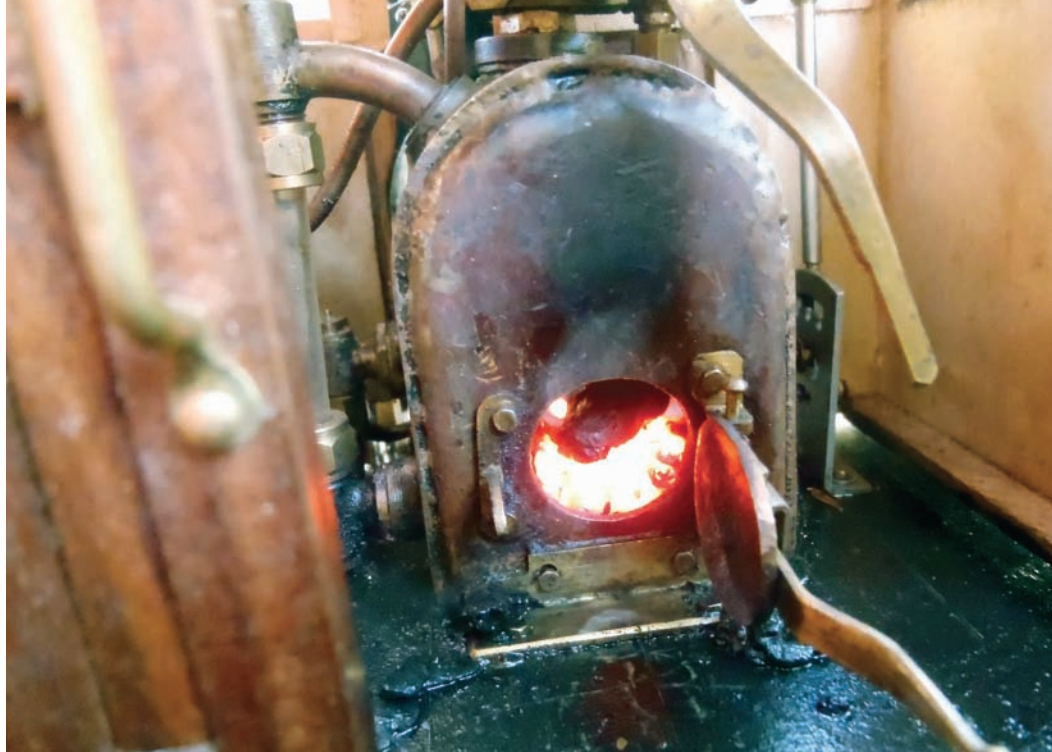
Test firing: The coal fire needs a good, deep bed of coals to burn well.
