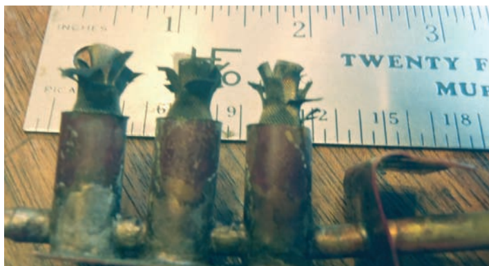
Alcohol: Left, the alcohol burner tubes were packed with various wick materials. Right, a wind-screen box reduces the amount of air drawn up into the fire box and increases the heat and efficiency of the burner.
