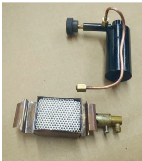
Butane burner: A ceramic burner was fabricated from a piece of perforated tile held in a copper box with a copy of 'Ruby's' burner tube and stock fuel tank and jet.
