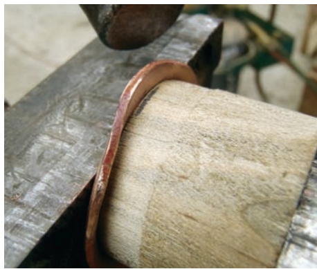
Tube sheet: Left, a disk of copper is cut for the front (end) tube sheet. Center, the copper was hammered into a cup shape around the hardwood form. Right, oversized tube sheet on form after the final hammering.
