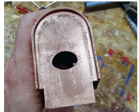
Boiler components: Left, the tube sheet being machined down for a snug fit on the boiler. Other pieces were made the same way; center, the throat piece, and right, the rear of the boiler fire box.
