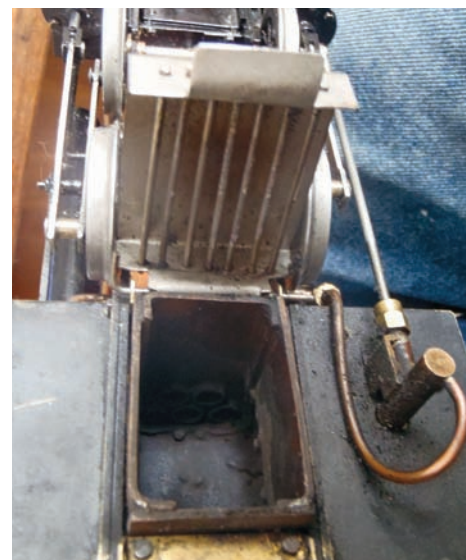
Second coal grate: An improved fire grate fits up against the bottom of the fire box, which gives a deeper bed of coal for a better fire (it's also easier to clean).
