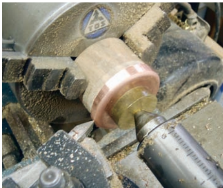
Boiler components: Left, the tube sheet being machined down for a snug fit on the boiler. Other pieces were made the same way; center, the throat piece, and right, the rear of the boiler fire box.
