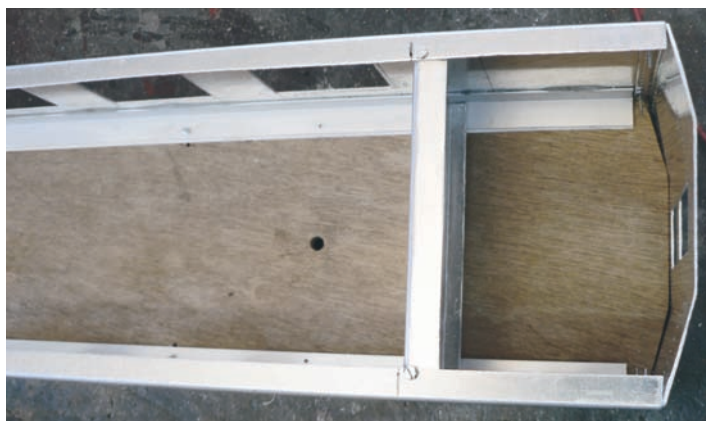
Support: On the D78 diner, an piece of angled aluminum is placed to provide strength.
