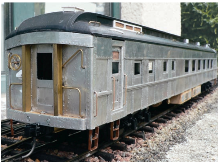
Details: Left, note the clerestory windows in the dining car's roof, the grab irons and steps; right, the roof's hatch on the end and the door.
