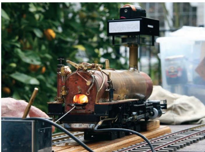
Test firing: The frame and boiler on the author's layout with temporary hoses attached to the tender.
