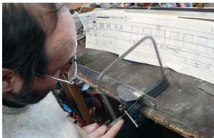
Doors, windows: Top, the D78's kitchen door has a spacer band to give it a recessed look. Bottom, the author uses his Bokfile (fret saw) to cut windows.
