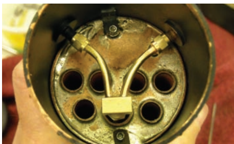
Photo 6: Inside smoke box, the T-box connects the super heater to two tubes that go to the flanges where pipes to engine will attach.
