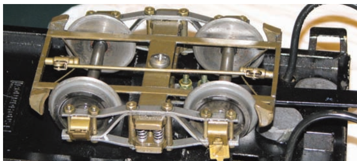
Mix-and-match: Accucraft arch-bar trucks (with Roundhouse wheels) on No. 24's tender.
