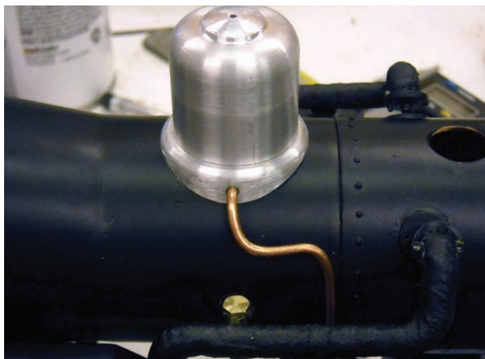
Photo 8b: Sand dome and piping are set in place. Note lagged steam pipe and clack valve below dome.
