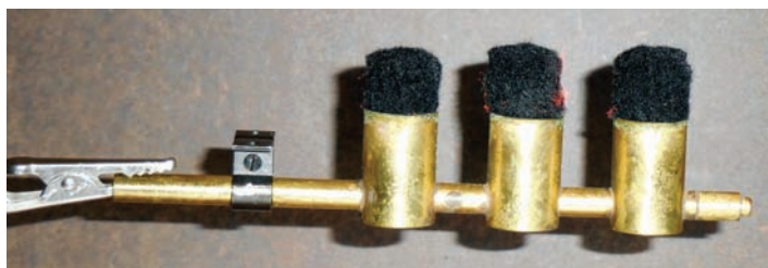
Photo 9: Pyron trimmed so that none of the wick material protrudes beyond burner tube sides.
