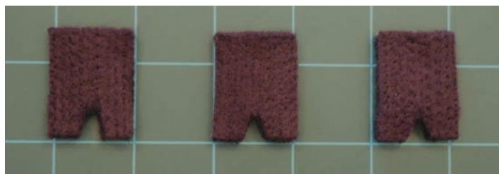
Photo 7: Pyron cut to enable material to be installed to reach the bottom of burner tubes.
