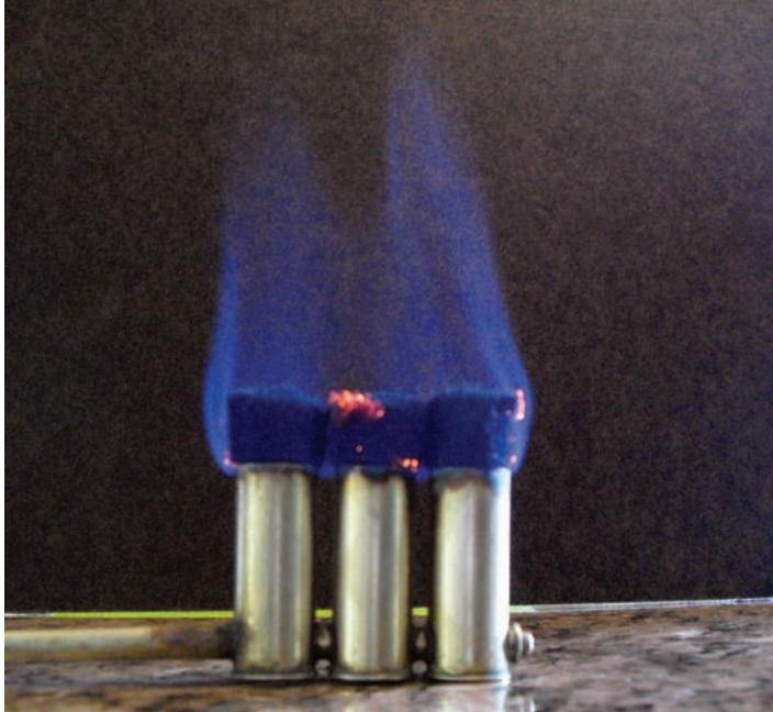
Photo 13: Untrimmed wicks for 'Spitfire.' Note short flame over the center wick.
