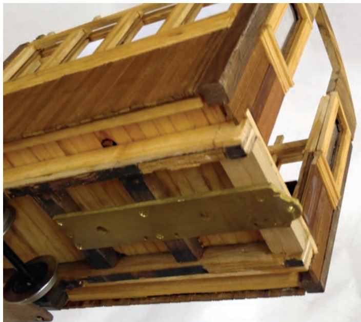
Coach coupler: A one-eighth-inch thick piece of scrap brass connects the coach to 'Dora's' coupler.
