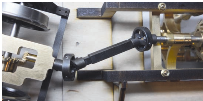
Geared: Drive shaft connects motor to wheels.
