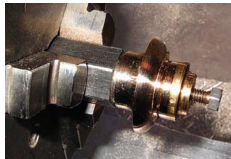
Chucked in lathe: Finished cap.
