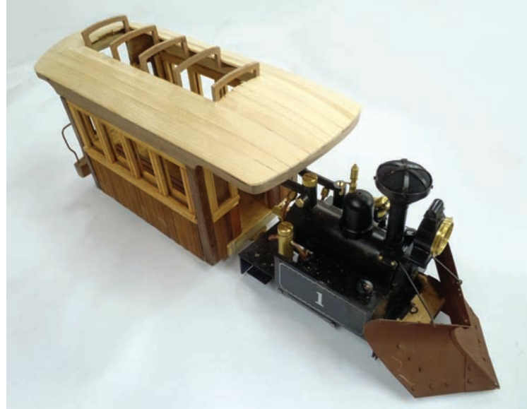
Top: Coach roof was extended forward to cover cab.
