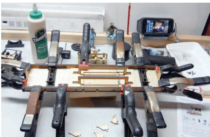
Glued: Frame and deck held together with clamps.
