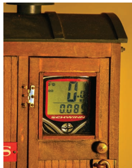
Seeing speed: Left, speedometer in a pocket in the car; right, the read out peeks through the car's door.
