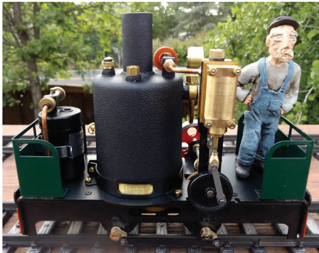
Oscillator: Single-cylinder drives a set of gears to propel 'Brunel.'
