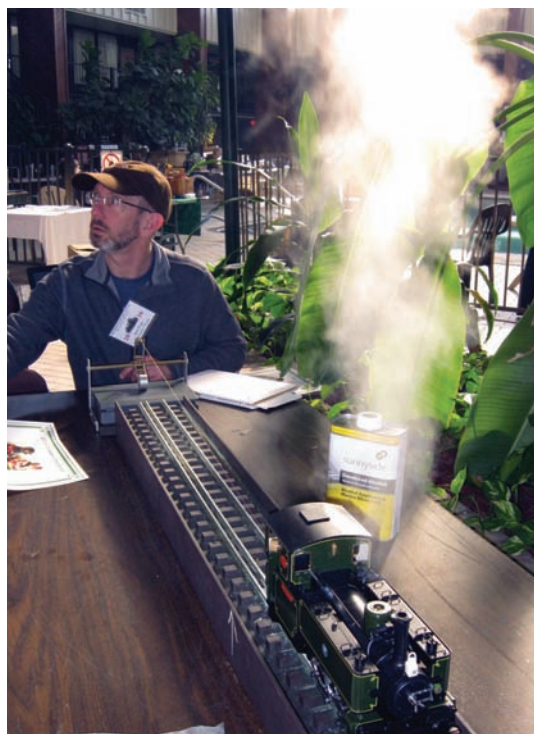
Testing: On the draw-bar pull rig, a Roundhouse supervised by Bob Pope.
