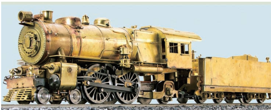
Pennsy E-6: Pilot model of Accucraft's new 4-4-2, without paint.
