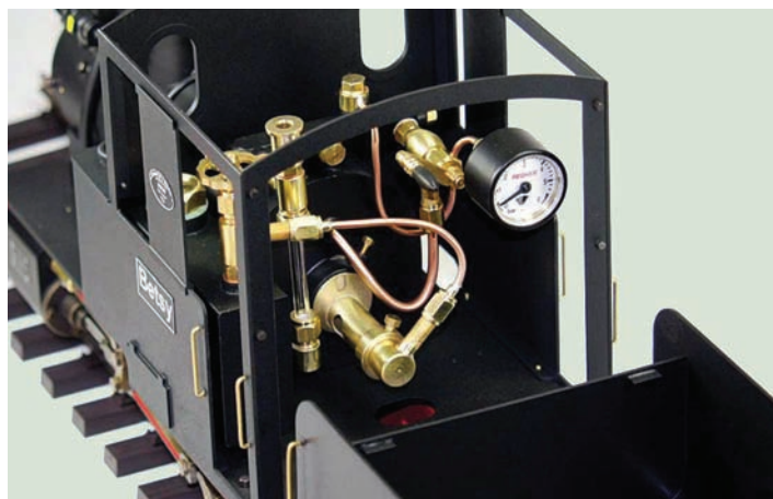
Regner 0-4-0: 'Betsy' kit is a butane-fired 1:22.5 scale locomotive in 45mm gauge.
