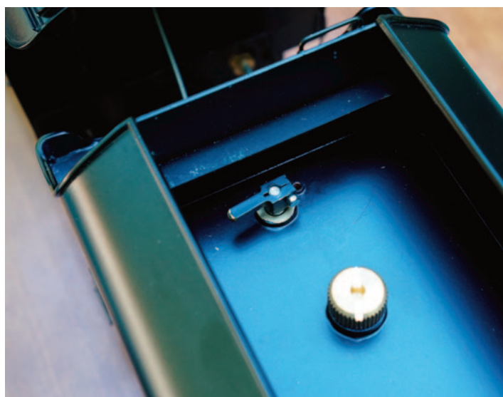
Photo 4: Coal load removed to show alcohol filler cap and valve.
