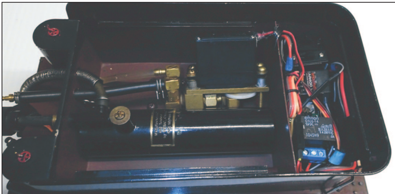
Photo 3 - Tender with wet and dry compartments and installed servo pump.
