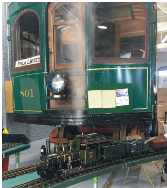
Shawe Coal-fired conversion of a Roundhouse Fowler gives off a nice plume as it passes one of the museum's trolleys.
