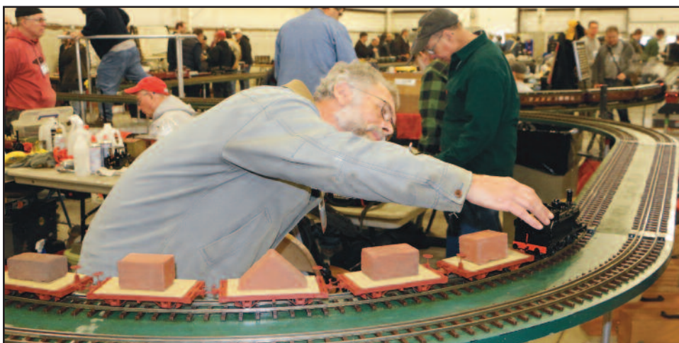
Henry Blanco-White puts his brand new Bowande-Wuhu 14xx locomotive through its paces on the small track at Cabin Fever. Henry uses the bricks not so much as a test load but a way to depress the cars springs so that the load rides smoothly. See Henry's review of the 14xx on page 22.
