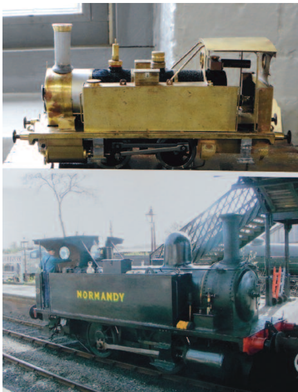
Another Ruby conversion – this one by Rob Kuhlman of Stowe, Pennsylvania. Based on an London and South Western Railway B4 class 0-4-0T dock tank project
