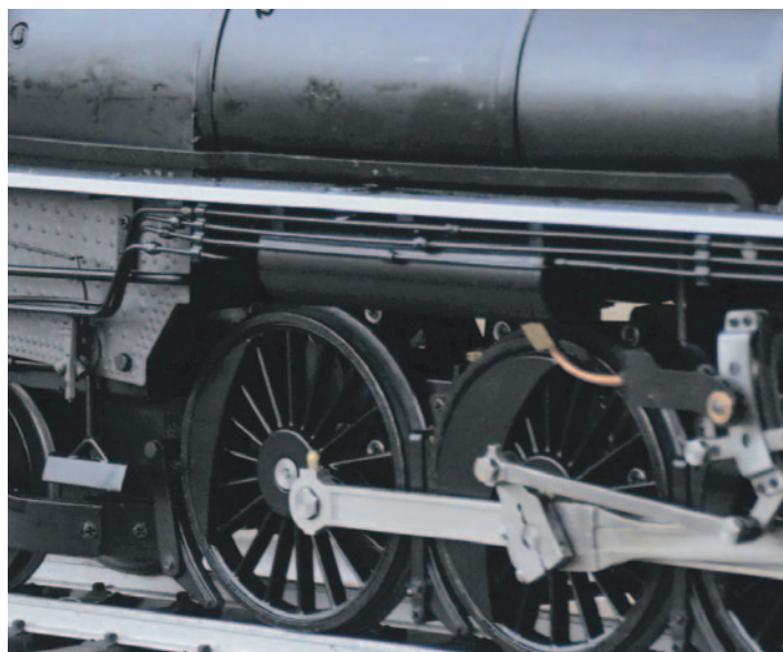
Deadleg oil reservoir tucked up under the right side running board.
